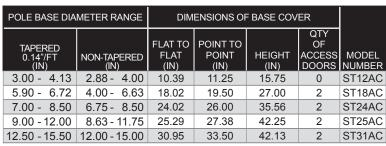
All dimensions shown are nominal and do not include handhole, baseplate or anchor bolt projections.
