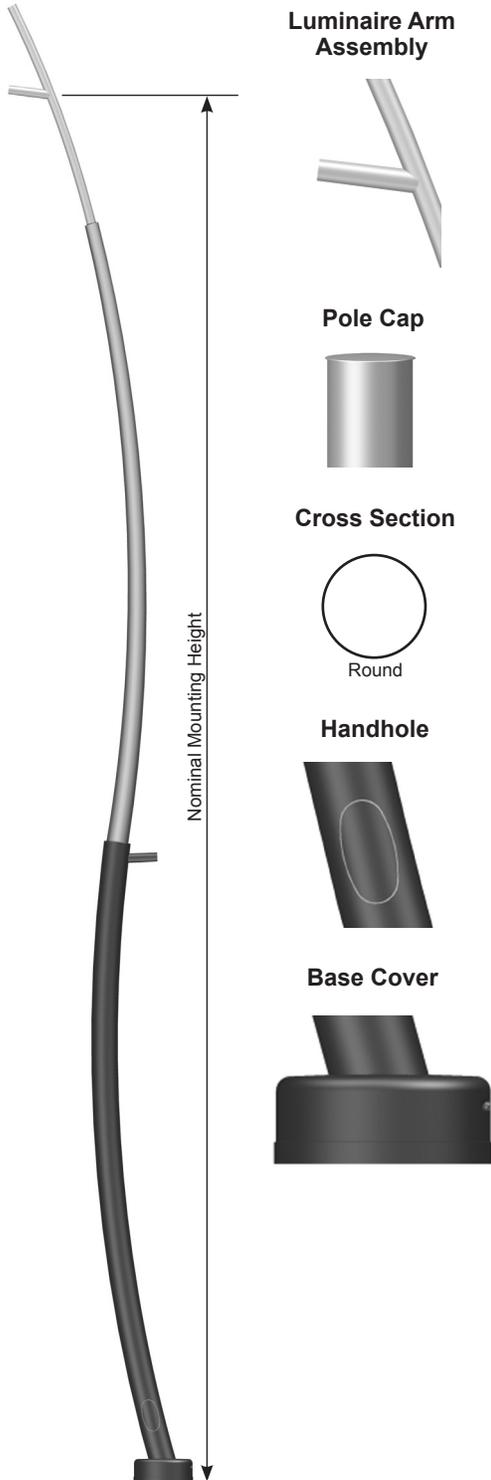
**Pole** - The pole shaft is spun from seamless alloy aluminum.
