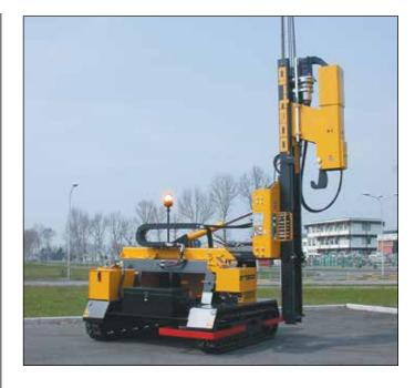
The self-propelled Ingal Smart Post Driver is specially designed for guardrail projects that require a manoeuvrable and easy to transport machine. A few simple commands move the machine from the 'shipping' position to the 'working' position reducing valuable set-up time.
