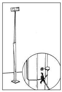
2. Remove allen keyed apron securing bolt.
