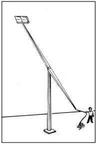
3. Pull apron away from stub section allowing the top section to gently swing downwards.
