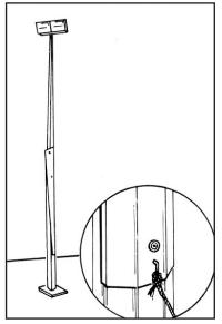
I. Fasten length of 12mm rope to the rope hook and secure.
