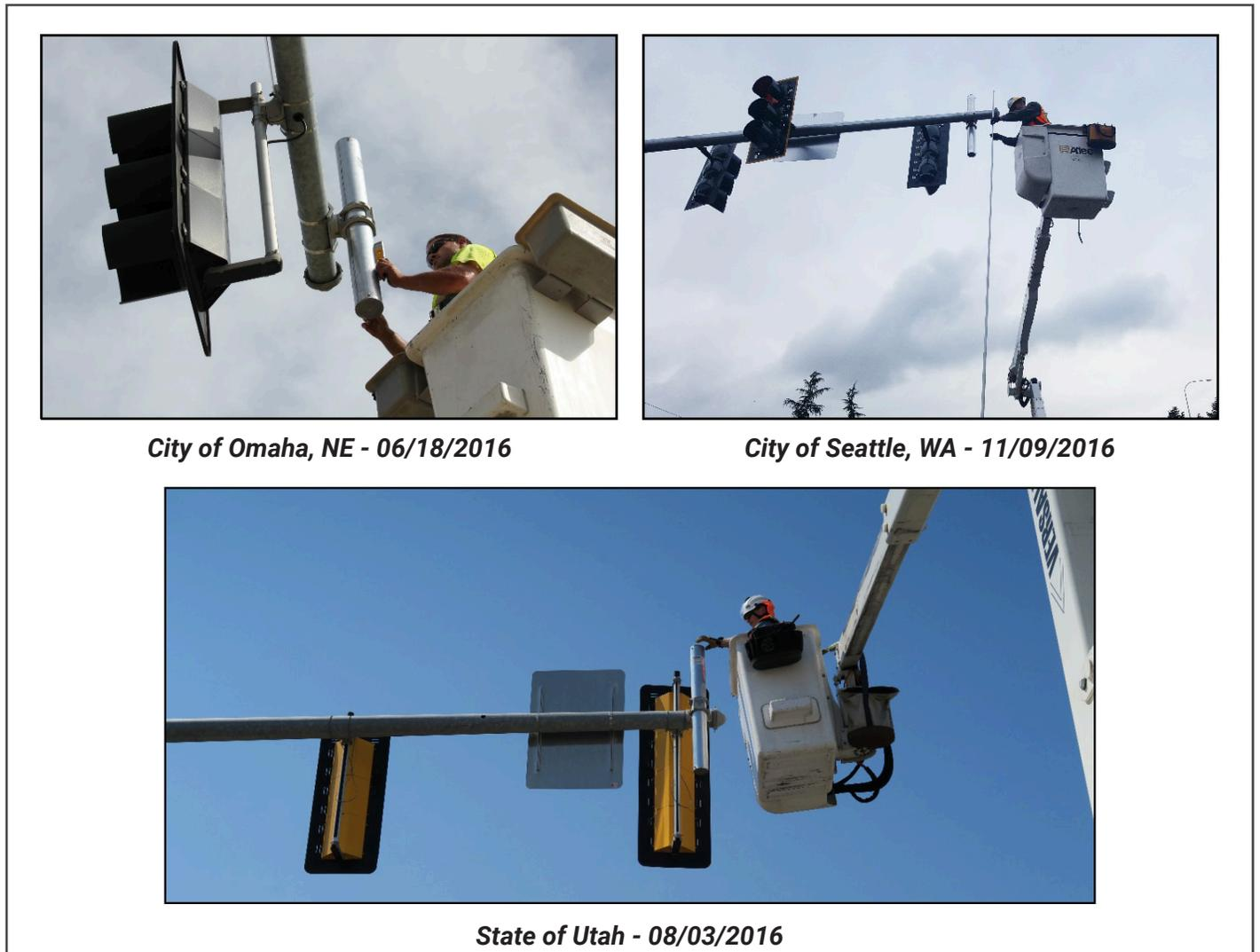
**Figure 5.** Free vibration (pluck) where performed at three different locations including the City of Omaha, NE, State of Utah, and the City of Seattle, WA.
