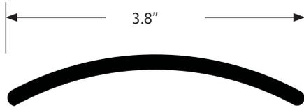
The GreenLine Single-Curve Marker is a highly flexible post featuring a simple, curved design that will take direct tire impacts at highway speeds. Decals or reflective sheeting can be applied to both sides. For hard soils, a convenient metal U-channel anchor may be added.
