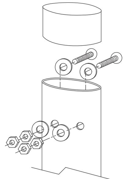
1/4" stainless steel round-head screws and hex nuts and nylon flat washers supplied, as illustrated.
