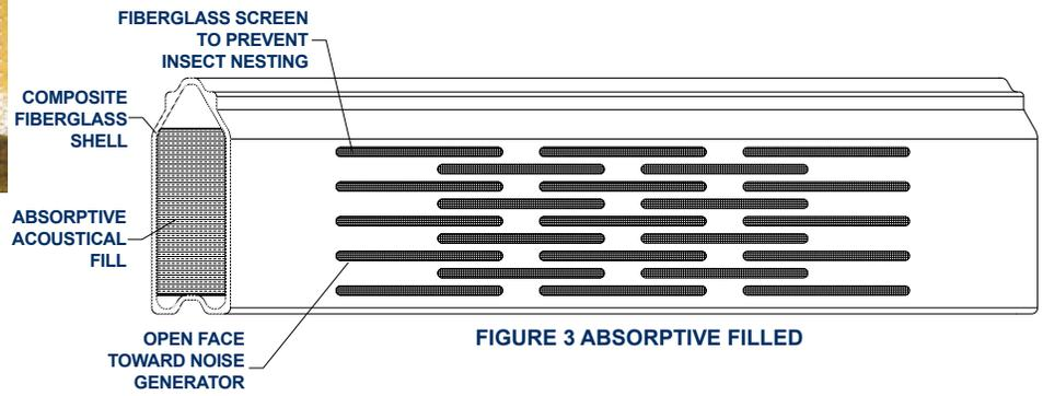
FIGURE 3 ABSORPTIVE FILLED
