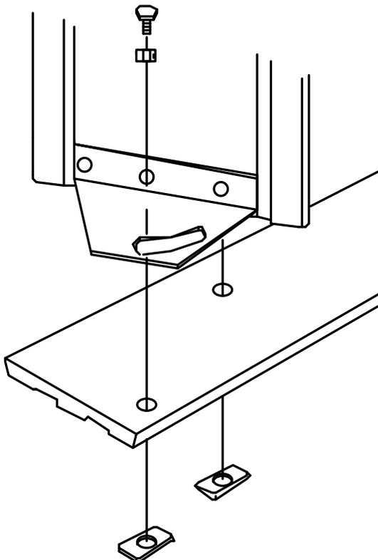
Blades can be attached to base rail before going on site.
