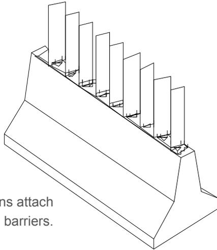
Modular sections attach easily to concrete barriers.
