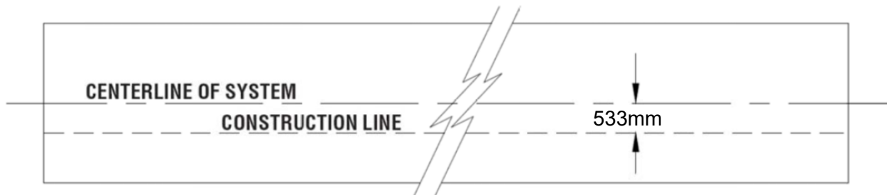
Figure 9 (Top view of foundation)
