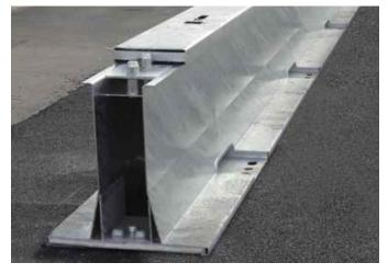
HighwayGuard<sup>™</sup> is the latest in innovative, portable workzone barrier technology. Symmetrical barrier sections with universal T-connector allows any section to connect to another, in either direction, significantly lowering installation time, operational costs and reducing inventory. A single truck, trailer mounted crane or excavator and crew can connect sections in less than 30 seconds, saving time and manpower.
