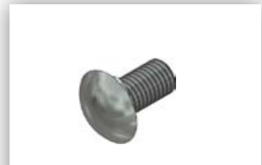
M16 x 32 Splice Bolt G8.8 ID: U PN: 3360G
