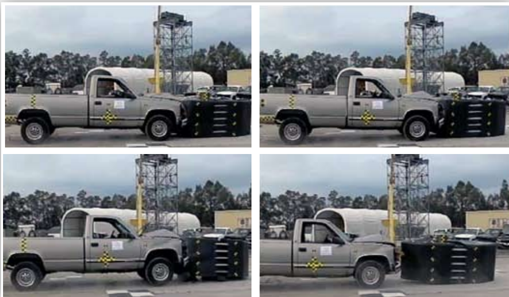
2000kg Pick-up truck impacting head-on with a pole using the RAPTOR™ at 50kph
