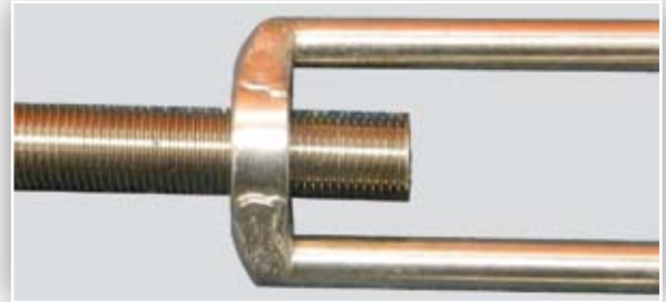
Figure 5: End Fitting Through Tension Fitting
