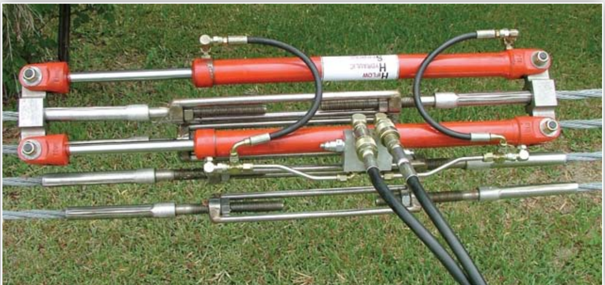
Figure 8: Tension Unit Connection to Tension Bay
