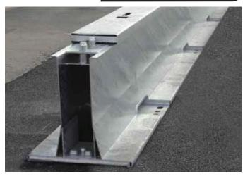
HighwayGuard™ LDS is a MASH 16 TL-3 compliant steel safety barrier. The 6m single barrier section, with the unique T-Connector provides quicker installation, removal and separation of barrier sections. It also offers the ability to remove sections within a run to create access gaps, replace damaged sections or alter barrier runs.
