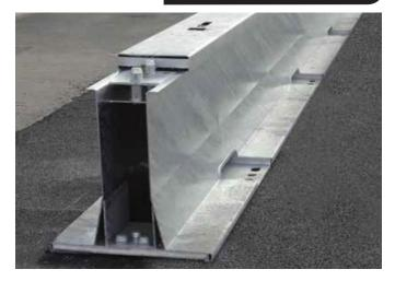
HighwayGuard™ LDS is a MASH 16 TL-3 compliant steel safety barrier. The 6m single barrier section, with the unique T-Connector provides quicker installation, removal and separation of barrier sections. It also offers the ability to remove sections within a run to create access gaps, replace damaged sections or alter barrier runs.
