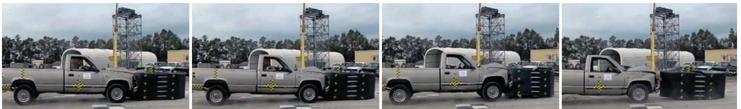
2000kg Pick-up truck impacting head-on with a pole using the RAPTOR™ at 50kph
