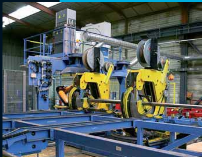
Soudage Semelle CN CN Flange Plate Welding
