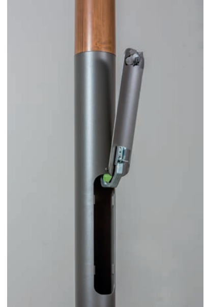
ALTO hinge fitted with a retractable end stop which allows the inspection door to be opened vertically and kept open. The system can be installed on all types of mast from ø 125 mm at the top of the door. Patented by Valmont Inc.
