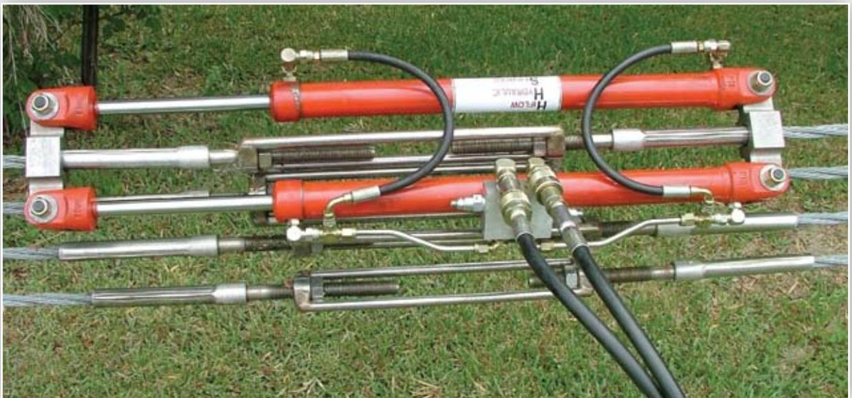
Figure 8: Tension Unit Connection to Tension Bay
