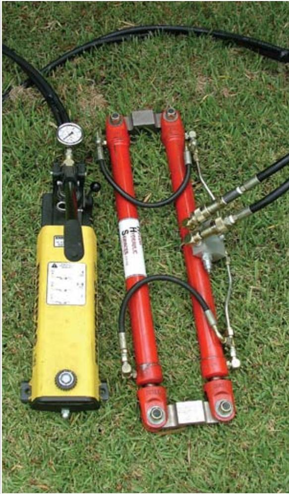
Figure 4: Hand Pump & Tension Unit
