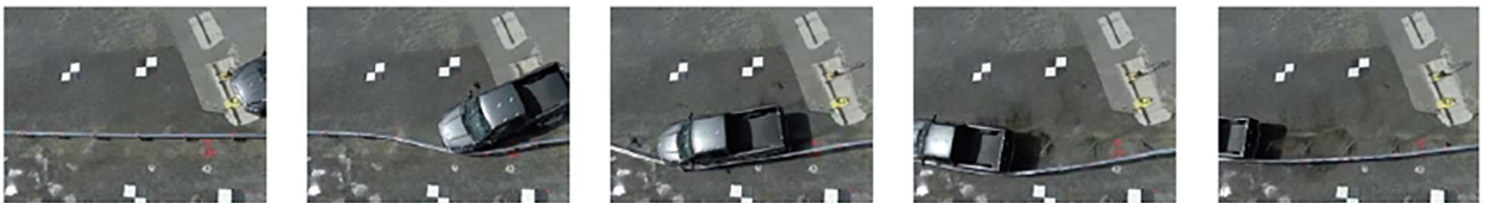
2270kg vehicle, 100kph, 25° Re-directive impact on EZYGUARD 4 (TEST 3-11 MASH)
