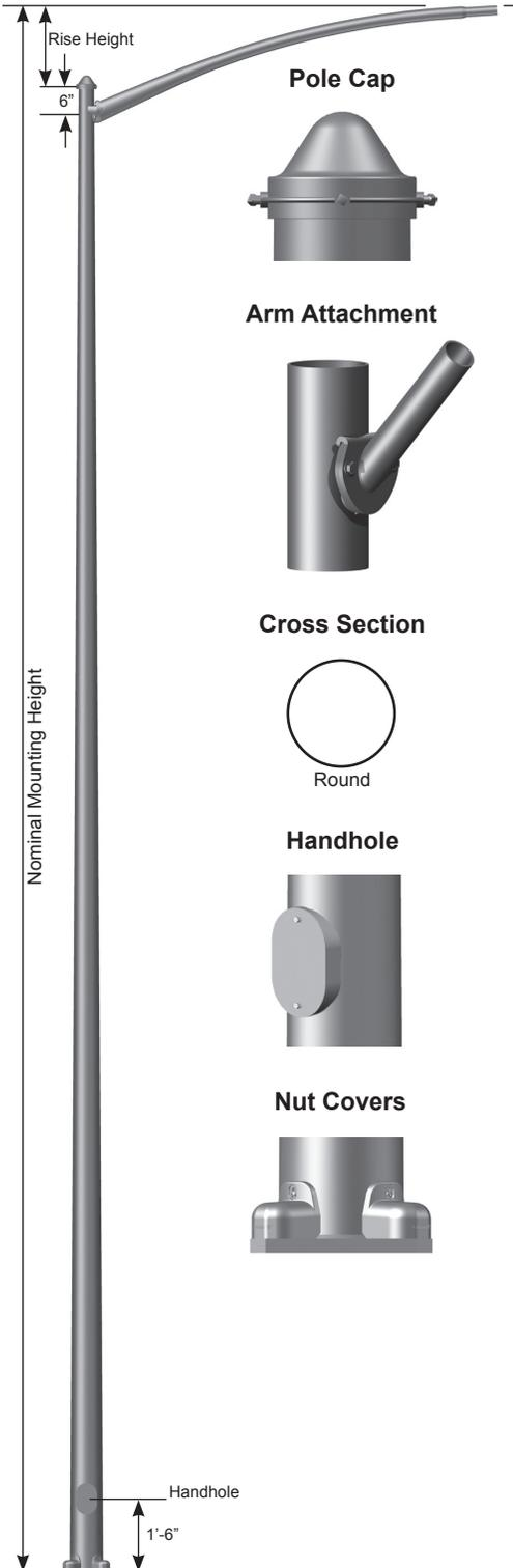
**Pole** - The pole shaft conforms to ASTM A595 Grade A with a constant linear taper of 0.14 in/ft.
